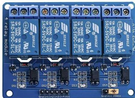
**Gambar 11. Modul Relay 4 Channel**
